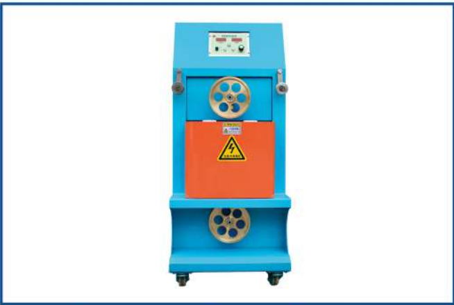
Copper wire preheater
